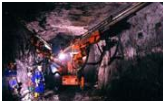
Twin-boom drill rig underground at Target
