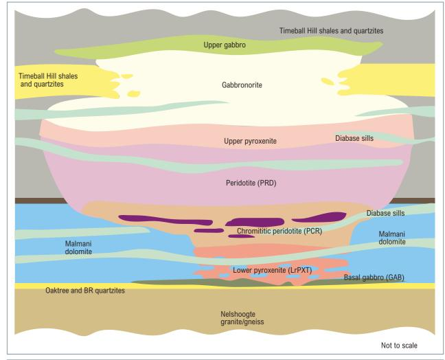
Legend Diabase Timeball Hill shale Massive chromitite Nelshoogte granite Klapperkop quartzite Upper gabbro Chromititic peridotite Rasement Rooihoogte formation Gabbronorite Lower pyroxenite Basal gabbro Malmani subgroup Upper pyroxenite Oaktree formation and black reef formation Peridotite (Harzburgite) **Uitkomst Complex** Transvaal Sequence
