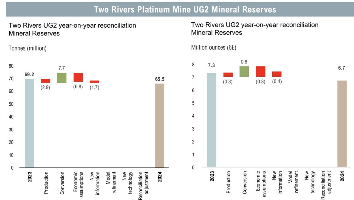
Mineral Reserves for the UG2 Reef decreased from 69.16 million tonnes at a grade of 3.30g/t (6E) to 65.32 million tonnes at 3.18g/t (6E) mainly due to mining depletions. A total of 2.9 million tonnes was depleted by mining. The UG2 Mineral Reserve 6E ounces decreased from 7.34 to 6.68 million ounces.
